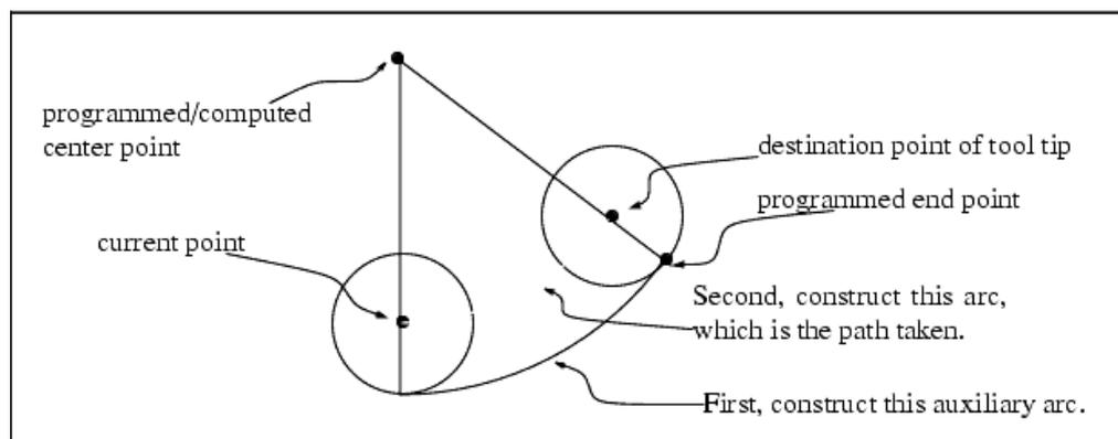
Figure A-7 shows the conceptual approach for finding the arc. The actual computations differ between the center format arc and the radius format arc (see Section 3.6.3).
