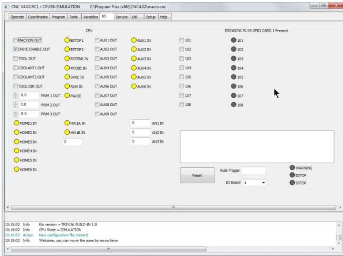
At this page you can monitor and set the I/O signals for CPU and IO extension board if attached. You can see that the GPIO extension board signals can be given a more meaningful name to your application. Note that this page shows the RAW IO values for the digital IO and does not take inversion into account.
