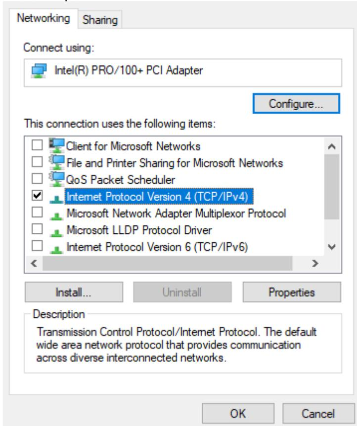
Switch on only TCP/IP V4 and uncheck the rest.
