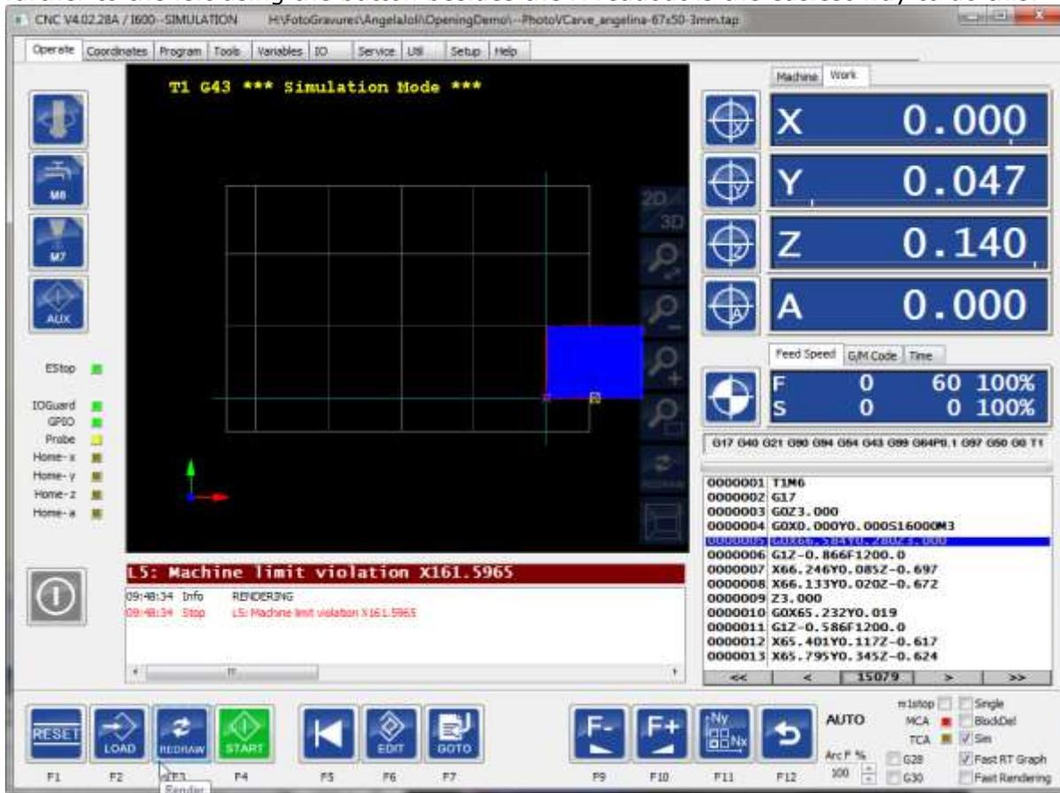
The yellow rectangle shows the first place where the collision is discovered. We see here clearly that a part of the tool-path is outside the machine area, a message is given showing the line number L5 in this case where the collision occurred. The easiest way to shift now is to jog to the place where you want to have the origin, the actual place of the work-coordinate system origin is shown as the cyan lines for X and Y.
