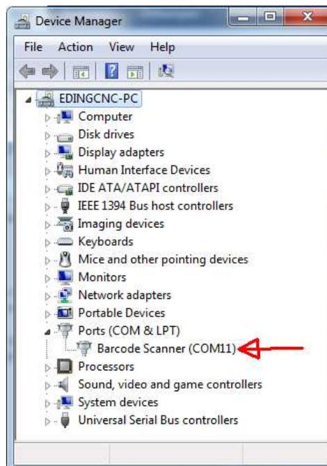
Some configuration is in the CNC.INI file, the device is connected with USB and can be seen in device manager as COMx port, this port number is set in the CNC.INI file under [USERINTERFACE]
