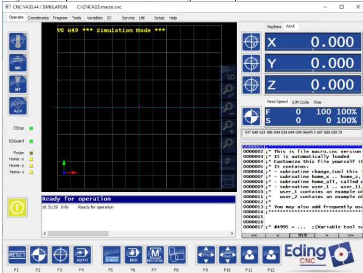
If all settings for your machine are correct you can press Reset (F1), this enables your drives. The buttons below are menu items, here the main menu (with company logo is shown). By pressing The F-Keys F2-F12 sub menus' with different buttons are shown.
