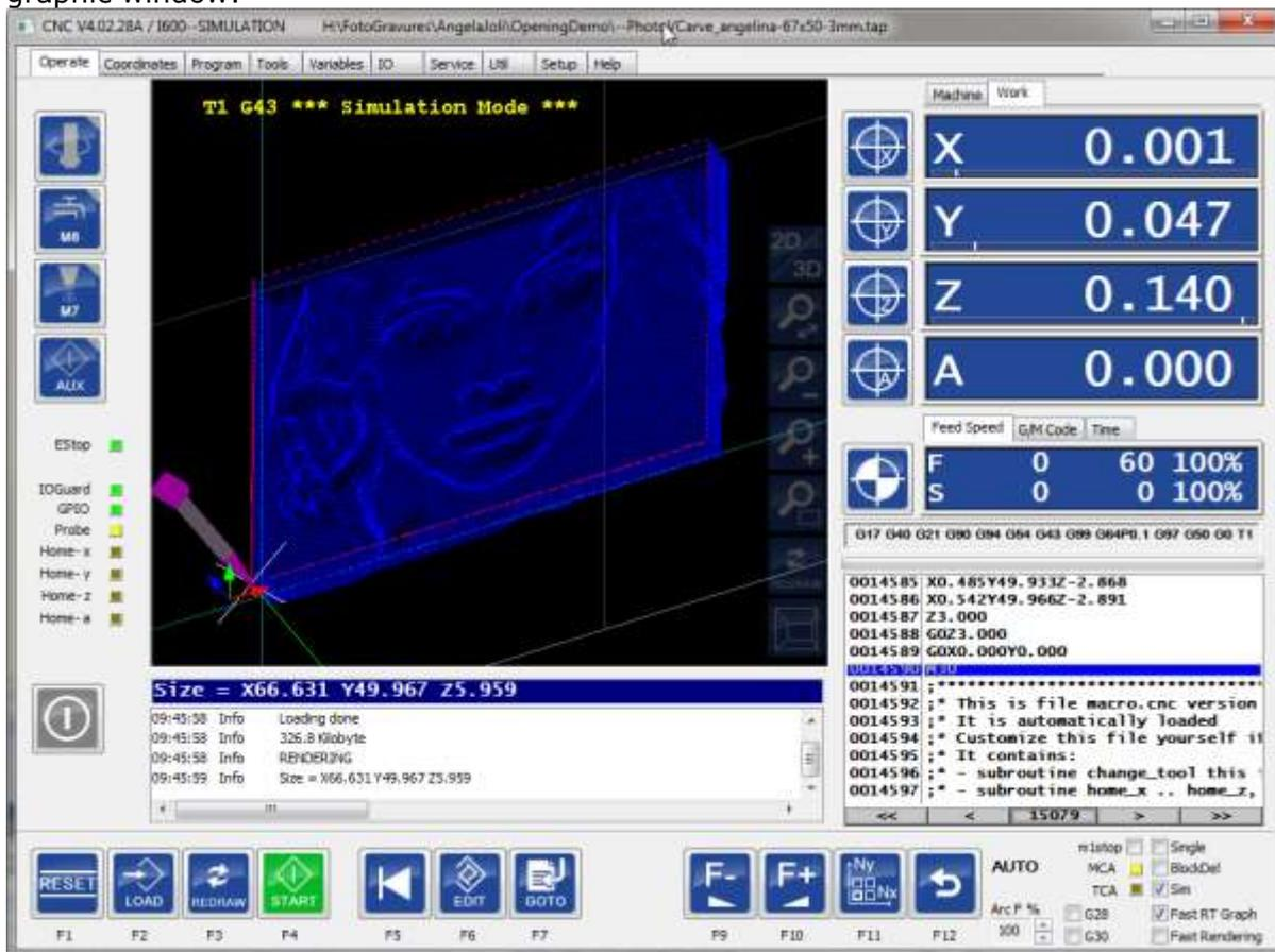
Using the mouse (ctrl+left mouse), you can rotate the tool-path and see it 3D.
