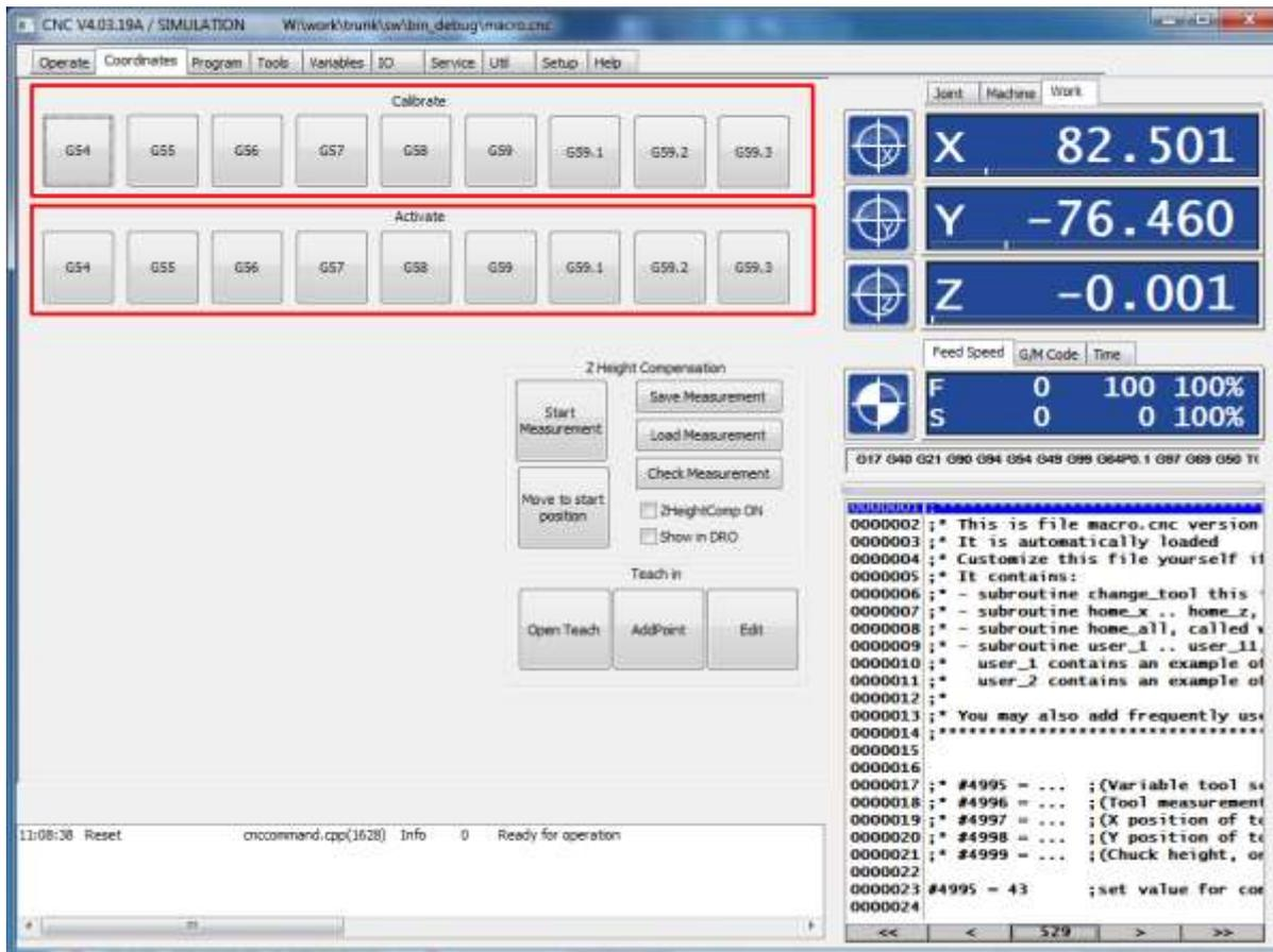
If you move to a position and press one of the calibrate buttons, the associated coordinate system offset (G54 – G59.3) is set such that the position becomes zero on this place when activated. See also G10 L20 P.. X.. Y.. Z.. because this is what is actually executed. Activation of one of the coordinate offsets can be done using one if the activate buttons, See G54 – G59.3.
