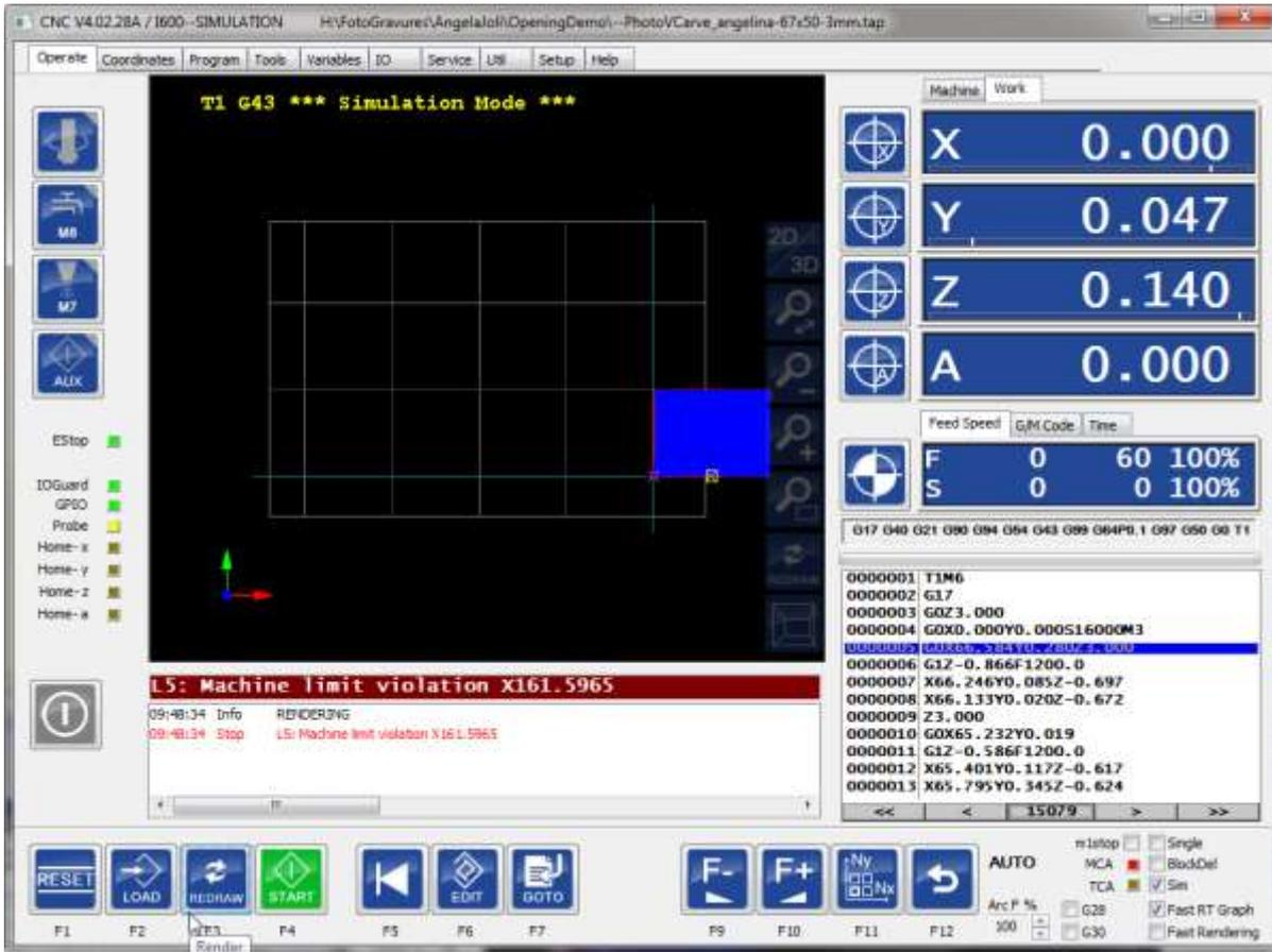
We see that the tool path fits without collision and we see the delta's in X, Y, Z, which is the size of the tool path.
