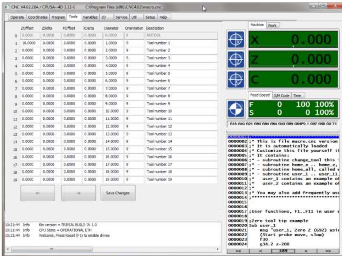
As you can see, there are additional parameters for turning, X-Offset X-Delta and Orientation.
