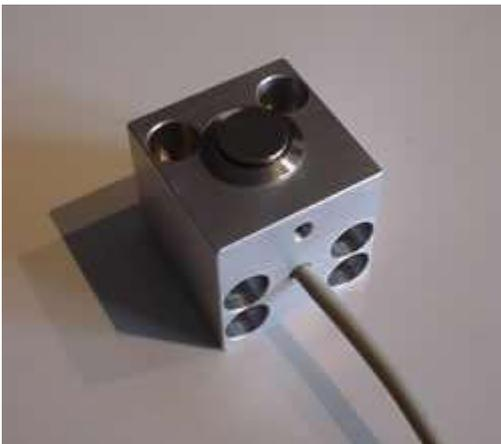
This routine calibrates the safe height, the XY position, the exact height of the tool setter. The positions are stored into persistent variables #4996 - #4999. The positions are used by subroutine m\_tool that is under user button 2.
