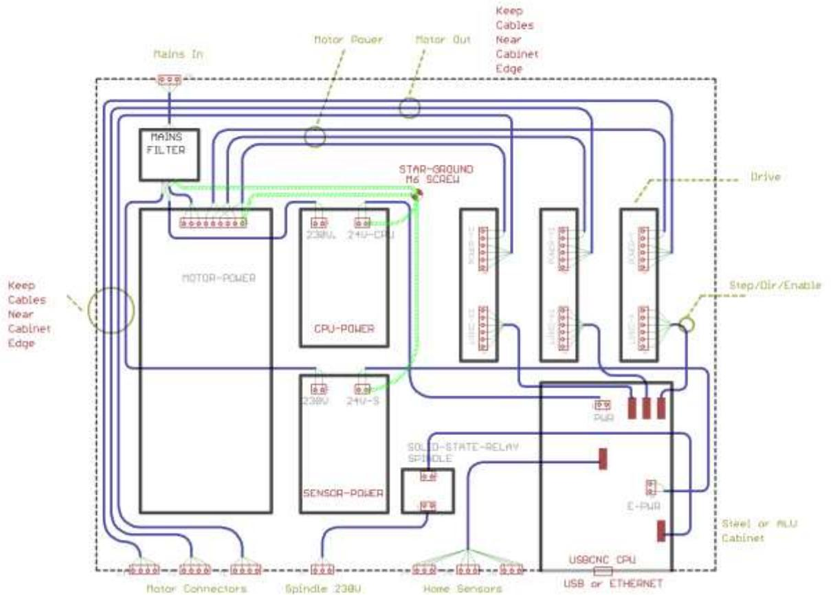
Here a picture of my own system, it contains various EMC problem makers, like 2 Switched mode power supplies and a frequency inverter for a HF spindle. Check the routing of the Motor and drive supply wires.
