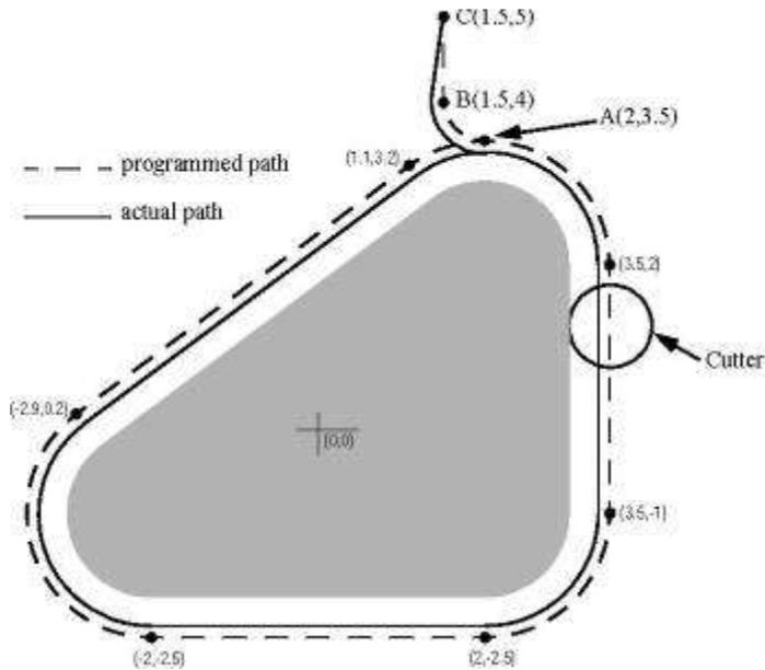
Cutter radius compensation is turned on after the first pre-entry move and before the second pre-entry move (including G41 on the same line as the second pre-entry move turns compensation on before the move is made). In the code above, line N0010 is the first pre-entry move, line N0020 turns compensation on and makes the second pre-entry move, and line N0030 makes the entry move.
