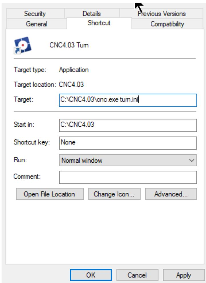
Add behind **C:\CNC4.03\cnc.exe** the name of the settings file to use for the software, in this case we use **turn.ini**. The result is that with the left **CNC4.03 Mill** Icon without changes except the name, **cnc.ini** is used as file name for all settings and with the right **CNC4.03 Turn** Icon, **turn.ini** is used for the settings. So now you have created 2 configurations. That is all.
