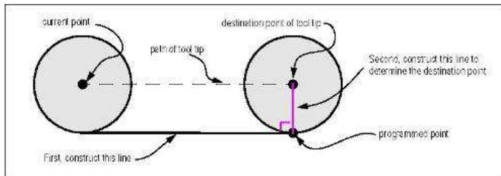
If the first move after cutter radius compensation has been turned on is an arc, the arc which is generated is derived from an auxiliary arc which has its center at the programmed center point, passes through the programmed end point, and is tangent to the cutter at its current location. If the auxiliary arc cannot be constructed, an error is signaled. The generated arc moves the tool so that it stays tangent to the auxiliary arc throughout the move. This is shown in Figure A-7.
