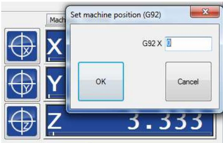
And you can also move the axes by holding the CTRL key and clicking with the left mouse button on the position display.
