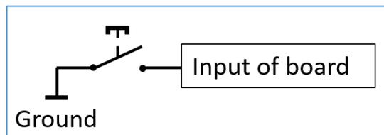
Figure 2 Switching HOME input in NPN mode.
