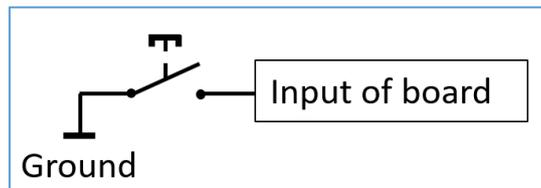
Figure 6 Connecting switch to PAUSE or RUN input.
