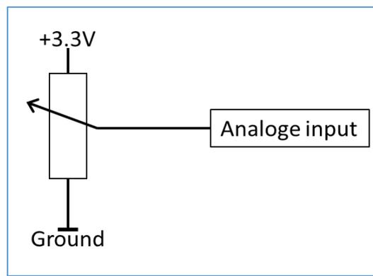
Figure 10. Connecting a potentiometer to the analogue input.
