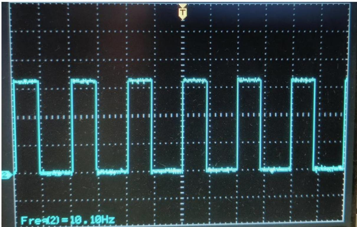
Figure 24 Charge Pump signal.
