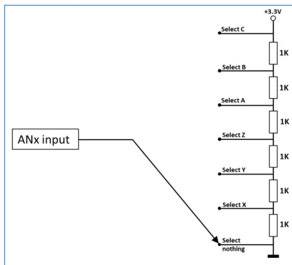
Figure 27. Selecting axis through an analogue input.
