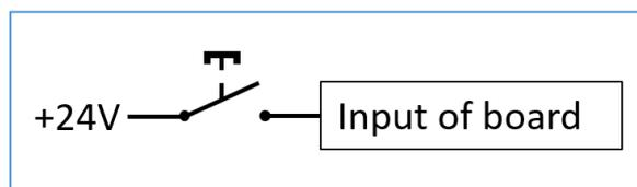
Figure 3 Switching HOME input in PNP mode.
