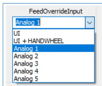
Figure 11. Setting up the analogue control of feedrate.
