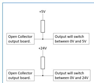
Figure 22 Creating different output levels with open-collector output.
