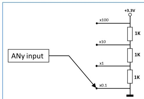
Figure 29. Selecting multiplication factor through an analogue input.
