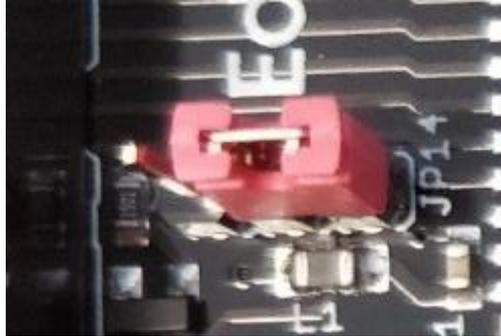
Figure 16. AUX output *shuts down* on E-STOP (default).
