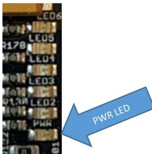
PWR: this LED indicates that the power for the processor is available (3.3V).
