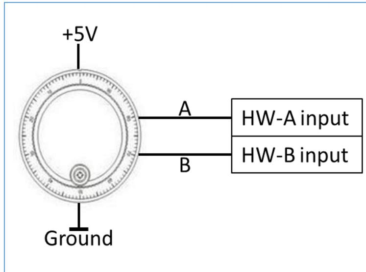
Figure 26. Connecting a handwheel.
