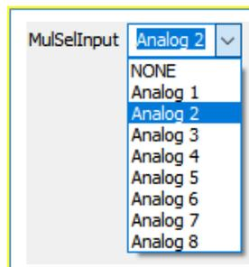
Figure 30. Selecting the analog input for the multiplier selection.
