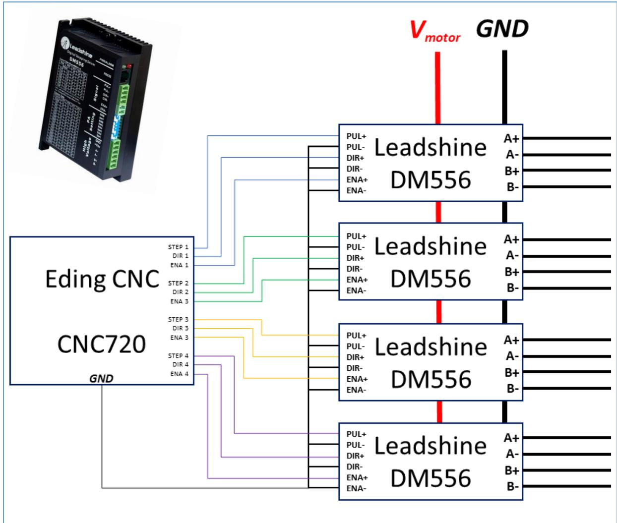
Figure 25. Diagram connecting CNC720 to Leadshine DM556 driver.
