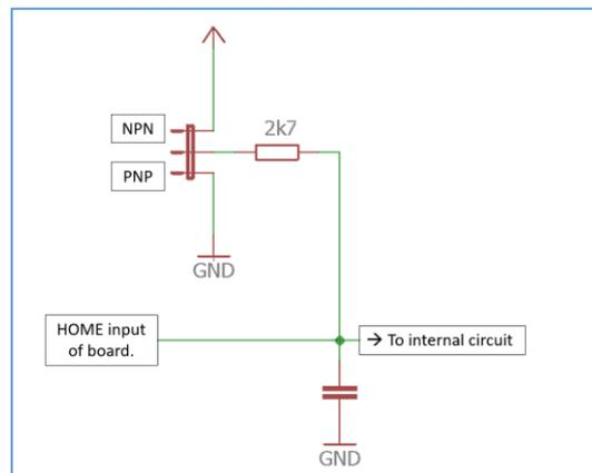
Figure 4 Input circuit of DRVALM input.
