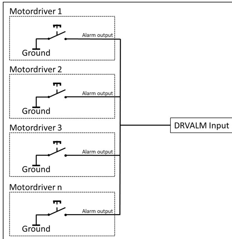
Figure 5 Combining open collector outputs of drivers.
