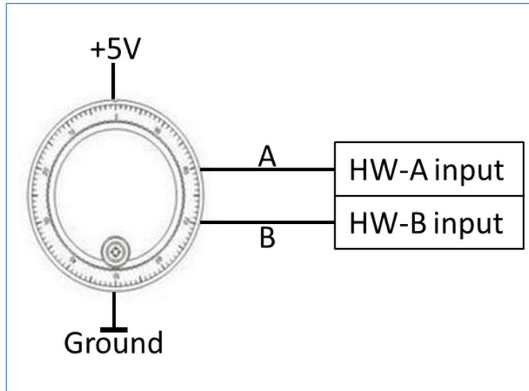
Figure 8. Connecting a pendant to the HW-A/HW-B inputs
