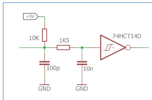
Figure 9 HW-A/HW-B digital inputs schematic.
