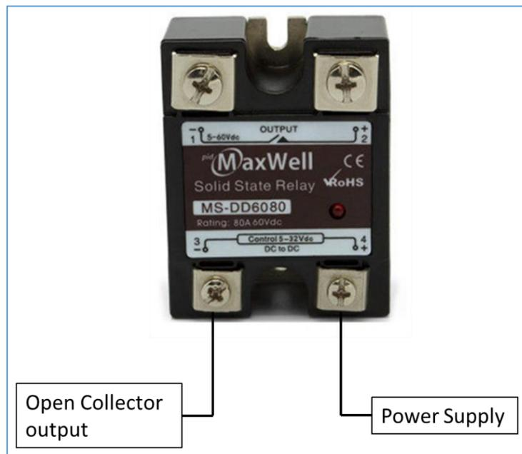
Depending on how the E-STOP hardware behavior is configured this output can be switched off in case of an E-STOP condition.
