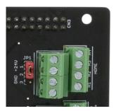
The jumper for the Estop Open Collector output can be set to 5V or 24V, depending on what type of relay you want to use. This voltage will be present on the '+' pin.
