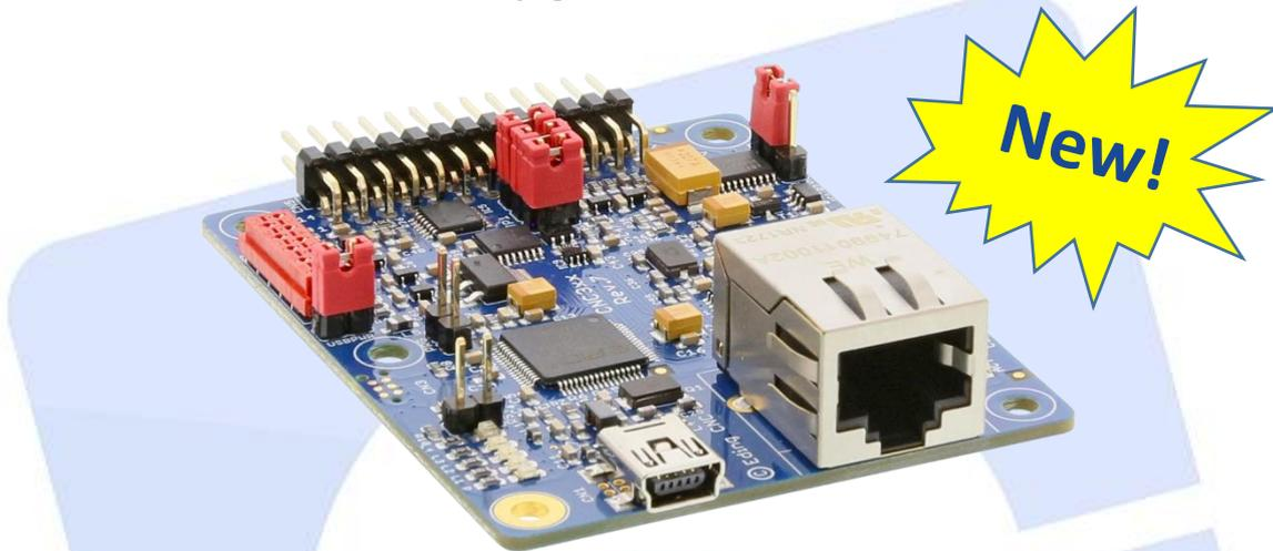
The smallest CNC controller from Eding CNC. This controller controls up to 3-axis with a 125kHz step frequency via its USB interface with Eding CNC Starter Software. This enables you to do 2.5D CNC operations. But wait...you need more?
