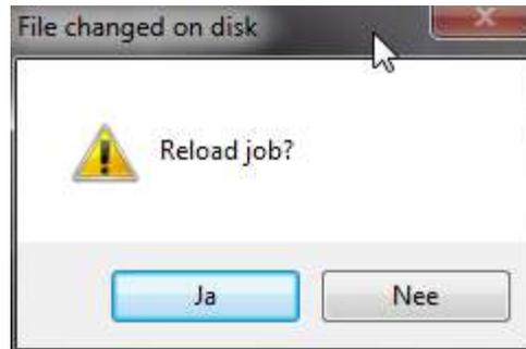
**load automatically:** If this is checked, the file is automatically loaded when it changes on disk, no dialog will appear.
