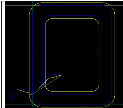
This example mills out a rectangular object from the outside and inside. On the outside we use G42, tool radius compensation right and for the inside G41, tool radius compensation left is used.
