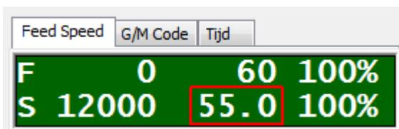
As you can see you can also choose to show an analogue input with a multiplication factor, this can be used when the spindle has a power used signal.
