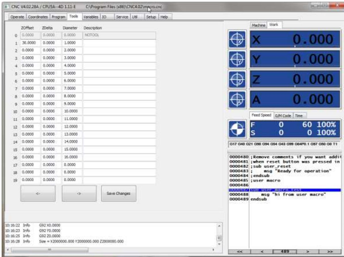
In this view you can define 99 tools with a Z-Offset(length) ZDelta (Delta due to Wear in Z length), diameter and description. The tool information is used when you use the tool radius and or tool length compensation functions of the G-Code interpreter commands (G40 – G43). See [chapter 3.6.](#) and further.
