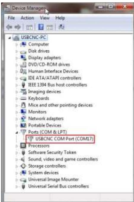
If you see this, the USB driver is correctly installed. The COM17 number may be different on your system.
