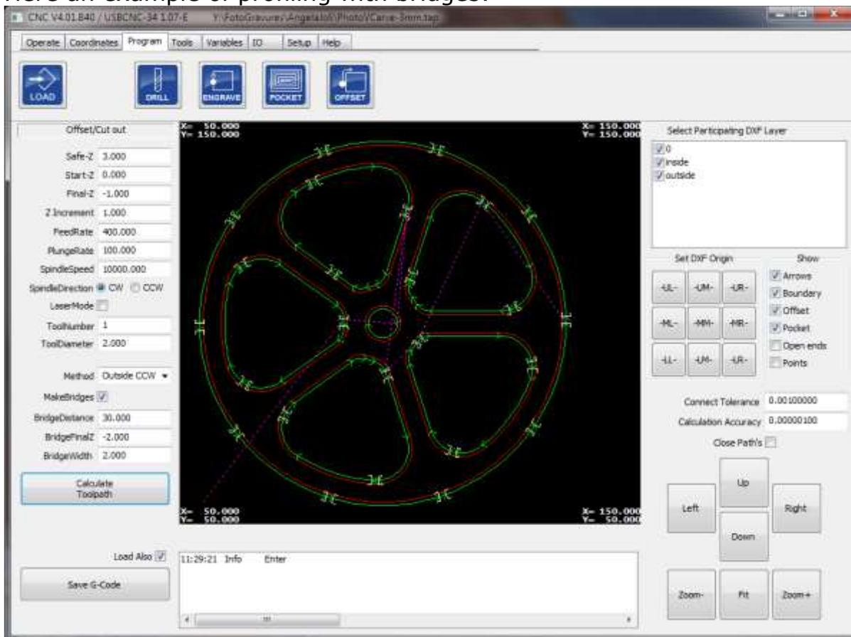
Note: The offset and pocket calculation might not always work, this is usually because of small errors in the drawing like lines over each other or not connecting lines. Experimenting with the Calculation Accuracy might help. Also check/correction of your drawing may help. The engraving function is robust and will always work.
