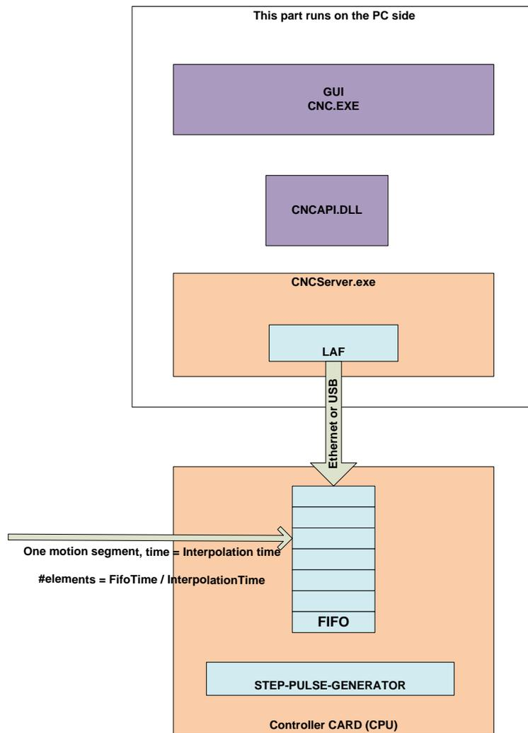
The **FIFO** makes it possible to perform smooth motion without hiccups on a non-real-time operating system like Windows. Because what happens is that sometimes Windows does things for itself for short times. This is no problem as long as the FIFO does not run empty. If the FIFO runs empty a **FIFO Underrun** error will occur.
