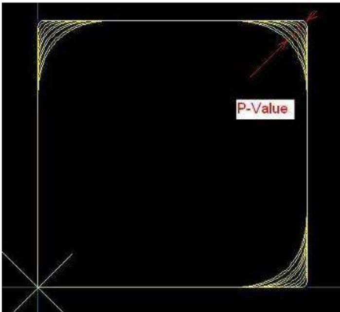
You may also conclude here that it is very important to have high acceleration on the machine because we can ramp down faster in the corner and have more accurate corners at higher speed.
