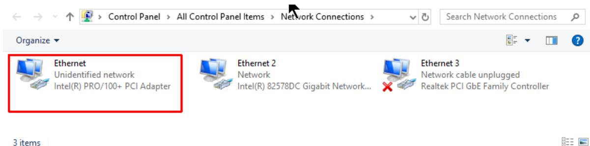
Double click the adapter card where the EdingCNC board is connected, you can recognize it because it shows "Unidentified network".
