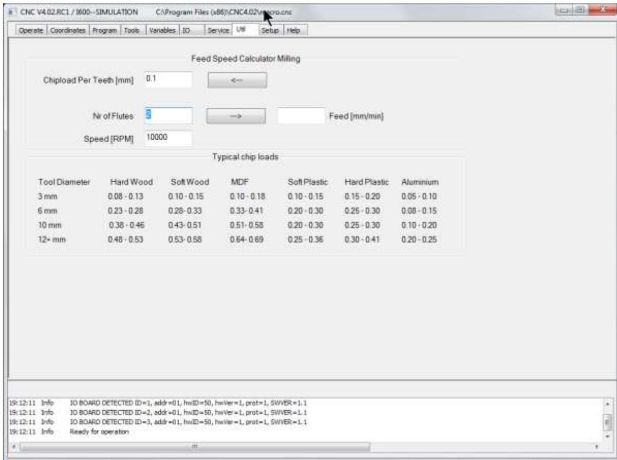
This page allows to calculate the right Feed/Speed for milling. Chip load is the quantity of material that is removed by one teeth of the milling tool. This is the most important parameter for calculating the feed given a Speed.
