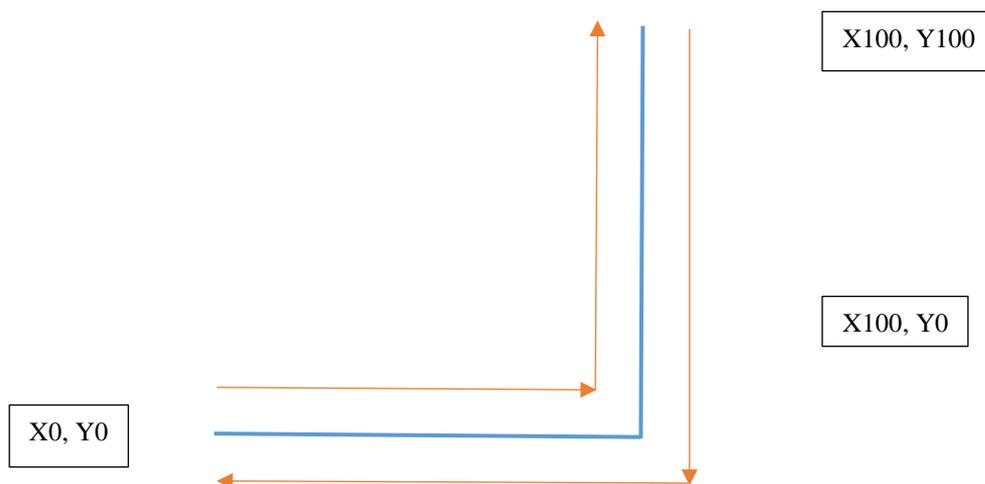
If we would make a move at Z1 (tanknife hi position), then the move would be the orange lines. With tanknife bend -1, the compensation is on the right side with respect to the move direction. On the other side with tanknife bend 1. The tanknife will automatically move up when the movement direction changes. The move up distance is specified in the setup. Also the angle at which a lift-up is required is specified in the setup.
