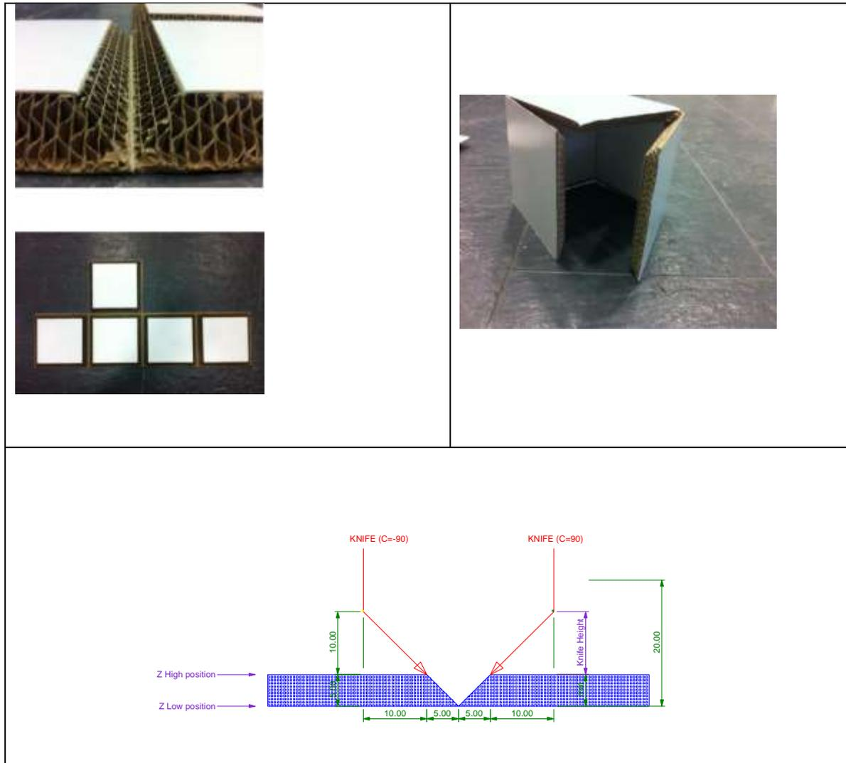
It is clear that with the bend knife during a z-move, the XY axes should move as well with same distance as Z, in the direction such that the sharp side of the knife moves under 45 degrees into the material. The user will program Z moves, the interpreter will rotate the knife (C axis) into the correct XY direction. Then kinematics will add the XY correction depending on the Z position.
