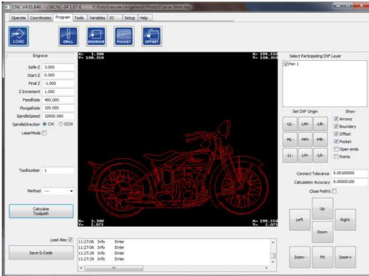
EDINGCNC uses a build in CAD/CAM library for these advanced import functions. You can load a file and then perform one of these operations:
