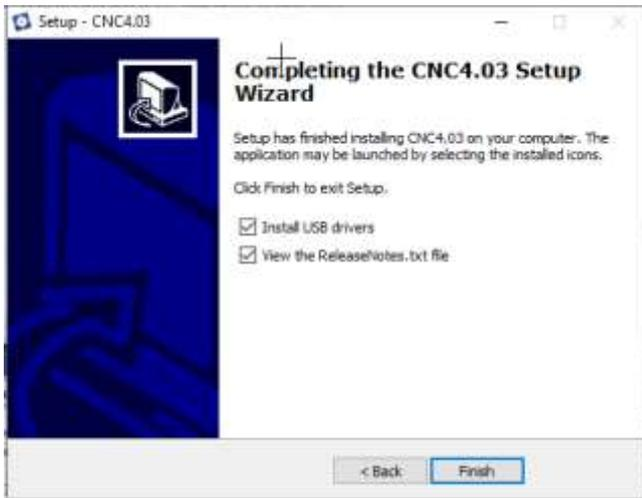
After installation reboot the PC, when it is rebooted connect the CPU, after 10 – 60 seconds, you will see that windows has found an EDINGCNC COM port if you are using and USB based CPU board. You can check that the USB driver is correctly installed in windows device manager, on windows 10, press windows key + X, then choose device manager.
