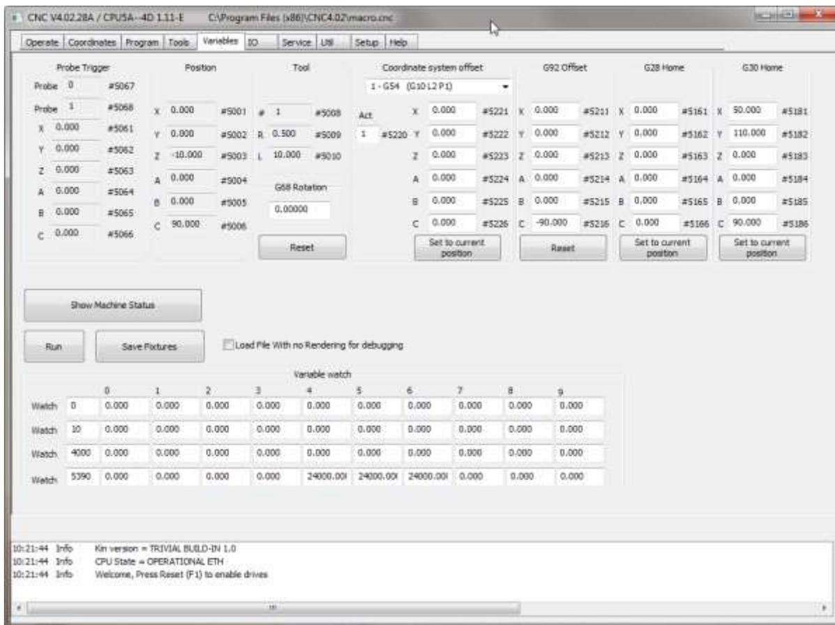
The G68 rotation can be reset with the reset button under G68 Rotation. This is the same as entering G69 in MDI.
