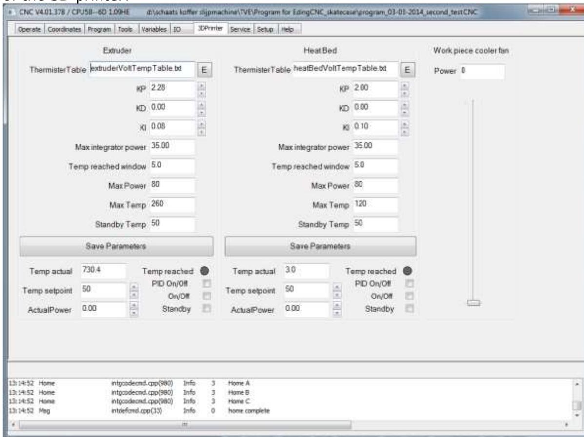
There are 2 equal parts for Extruder and Heat bed control and a slide to adjust the cooler Fan for the work piece. The temperature is read from analog inputs of the CPU and the Heat and Fan power is controlled by PWM outputs.
